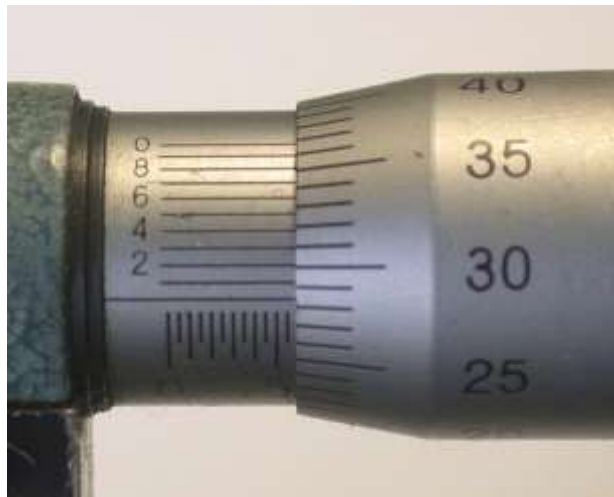
Fig 01-08: Micrometer with a vernier scale. Vernier micrometer reading 5.783 \text{ mm} \pm 0.001 \text{ mm} . made up from 5.5mm on main screw lead scale, 0.28mm on screw rotation scale, and 0.003mm added from vernier.
