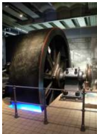
Fig 2.26: Flywheel of a steam engine in a factory
