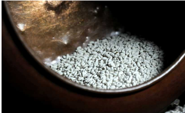
Fig 3.19: Candy being panned (coated) in a giant pot at a candy factory in Nablus, West Bank https://commons.wikimedia.org/wiki/File:Candy_in_the_making_in_Nablus_027_-_Aug_2011.jpg#/media/File:Candy_in_the_making_in_Nablus_027_-_Aug_2011.jpg
