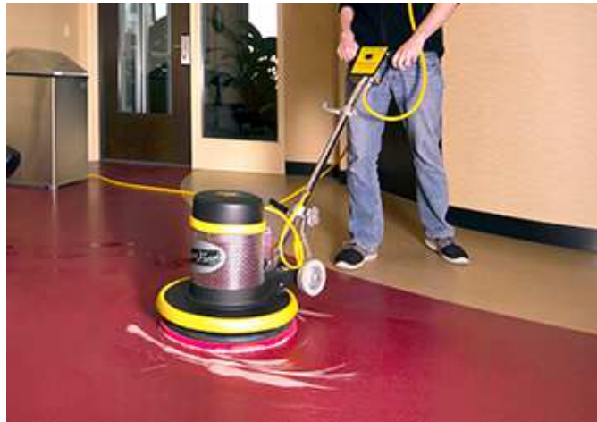
Fig 1.11: Spray buffing on floor
