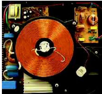
Fig 1.00: Inside view of an induction cooker: the large copper coil forms the magnetic field, a cooling fan is visible below it, and power supply and line filter surround the coil. In the centre of the coil is a temperature sensor, covered in white thermal grease
