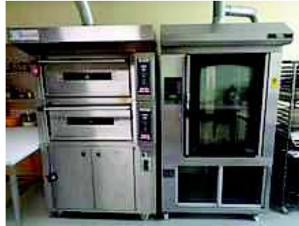
Fig 1.00: Industrial "Zanolli" double hearth deck oven (left) and "Sveba-Dahlen" rotary rack oven (right) at the Faculty of Food Technology, Latvia University of Agriculture bakery
