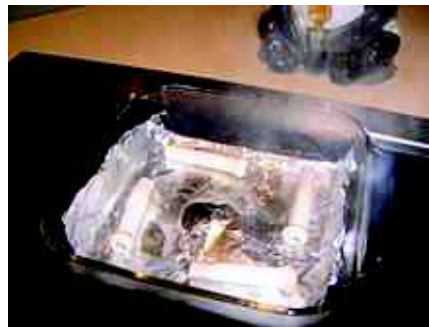
Fig 1.00: Household foil is much thinner than the skin depth in aluminum at the frequencies used by an induction cooker. Here the foil has melted where it was exposed to the air after steam formed under it. Cooking surface manufacturers prohibit the use of aluminum foil in contact with an induction cooking surface.
