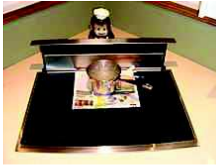
Fig 1.00: An induction cooking surface boiling water through several layers of newsprint. The paper is undamaged since heat is produced only in the bottom of the pot
