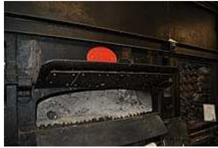
Fig 3.00: Manlove, Alliott & Co. Ltd. 1894 destructor furnace. The use of incinerators for waste disposal became popular in the late 19th century.
