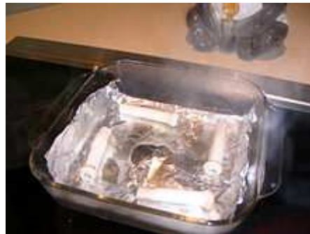
Fig 1.00: Household foil is much thinner than the skin depth in aluminum at the frequencies used by an induction cooker. Here the foil has melted where it was exposed to the air after steam formed under it. Cooking surface manufacturers prohibit the use of aluminum foil in contact with an induction cooking surface.
