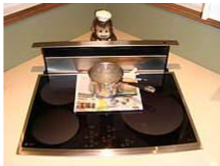
Fig 1.00: An induction cooking surface boiling water through several layers of newsprint. The paper is undamaged since heat is produced only in the bottom of the pot
