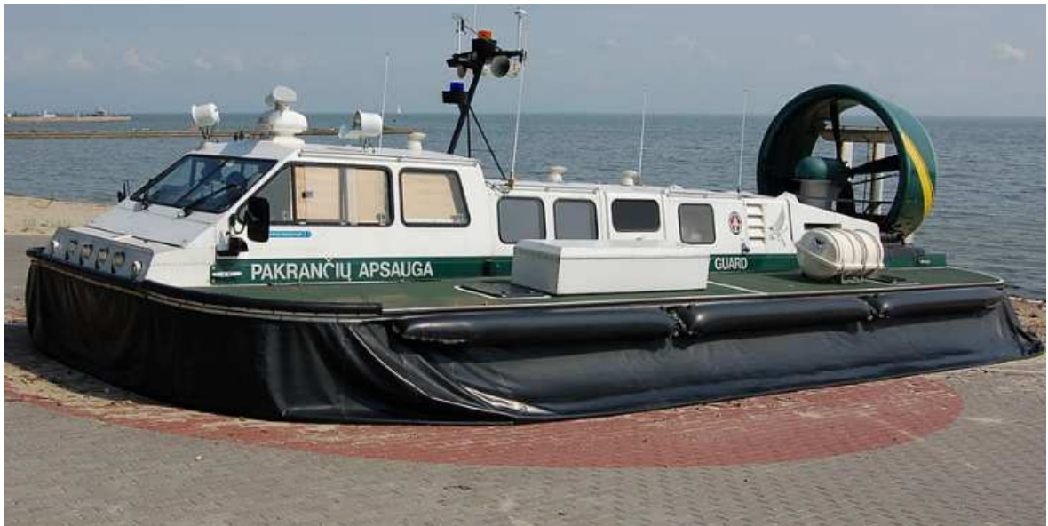
Fig 4.16: A Lithuanian Coast Guard hovercraft with engine off and skirt deflated
